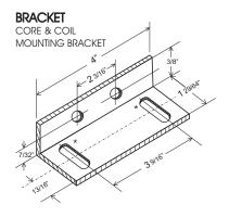
1353 Mounting bracket for Core & Coil Ballasts (1 bracket with thru bolts) \* 1⁄4" x 11⁄4" 2 SLOTS
